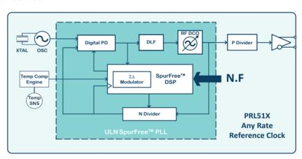
**PRL51X** supports XO, VCXO and DCXO Modes, Single, Dual, Quad and Any-Rate (I2C) Modes and a tight temperature stability option with a  $\pm 3$  ppm (-40 - +85 °C).
