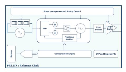
**PRL21X** supports XO, VCXO and DCXO modes, Single, Dual, Quad and Any-Rate (I2C) configurations while exhibiting low phase noise with a typical integrated RMS Jitter of 350 fs for any frequency up to 1 GHz.
